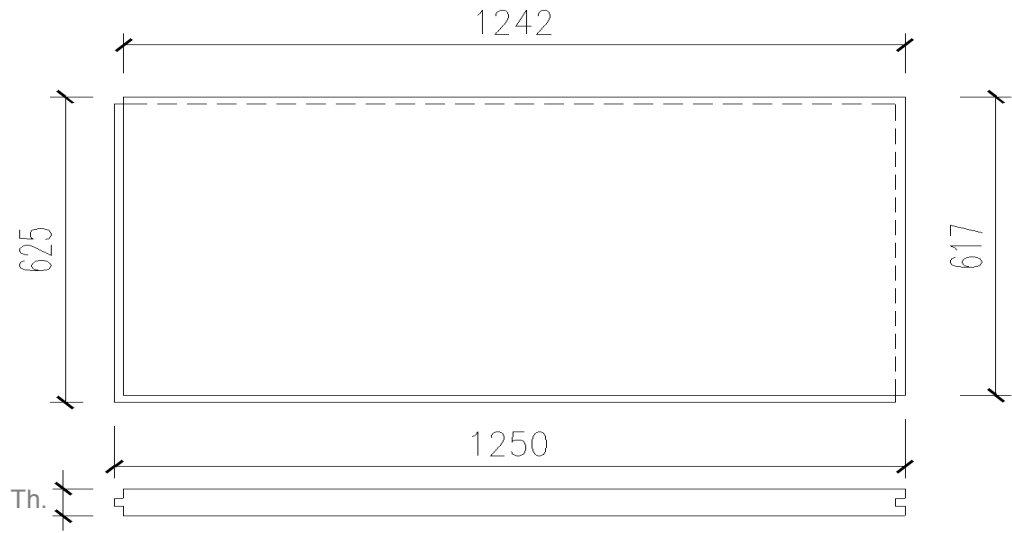
Board size for types PD and PDB, without tongue – 617 x 1242mm
